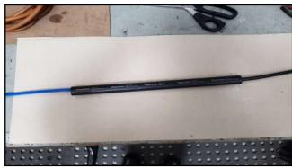
Start shrinking in the middle of the sleeve and then working out to the ends.
